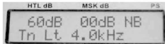
Fig. 7.8. Microcontroller based audiometer with 2 row LCD display.
