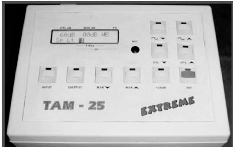
Fig. 7.8. Microcontroller based audiometer with 2 row LCD display.
