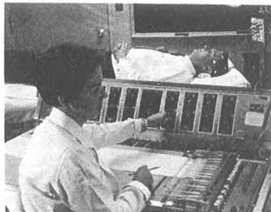
(b) A switch selector allows the desired electrode configuration to be chosen.
