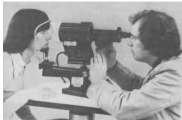
Fig. 7.17b. The Keratometer for prescribing lens (a) principle.
